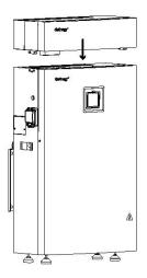
Step10: Connect MPPT Unit to All in One II with screws
