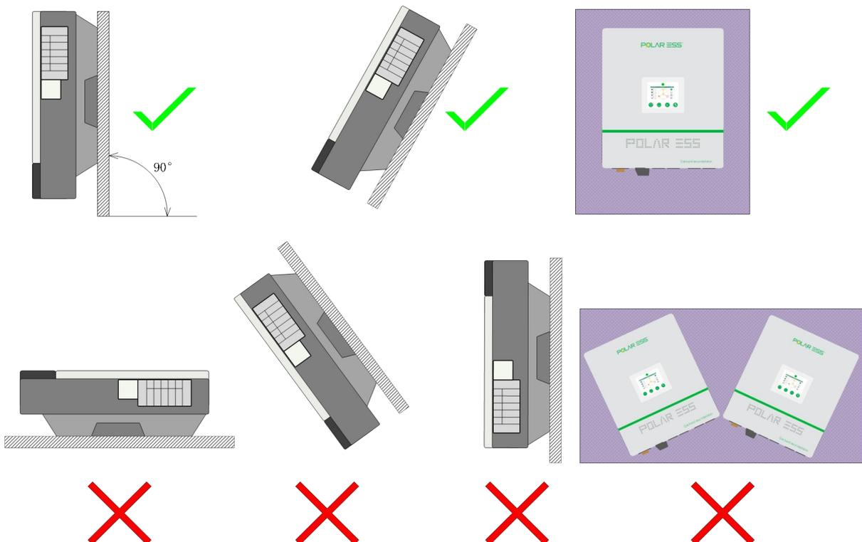
The inverter should not be installed in direct sunlight, direct heavy water sources or unstable locations. We recommend that the inverters be installed at a location with some cover or protection.
