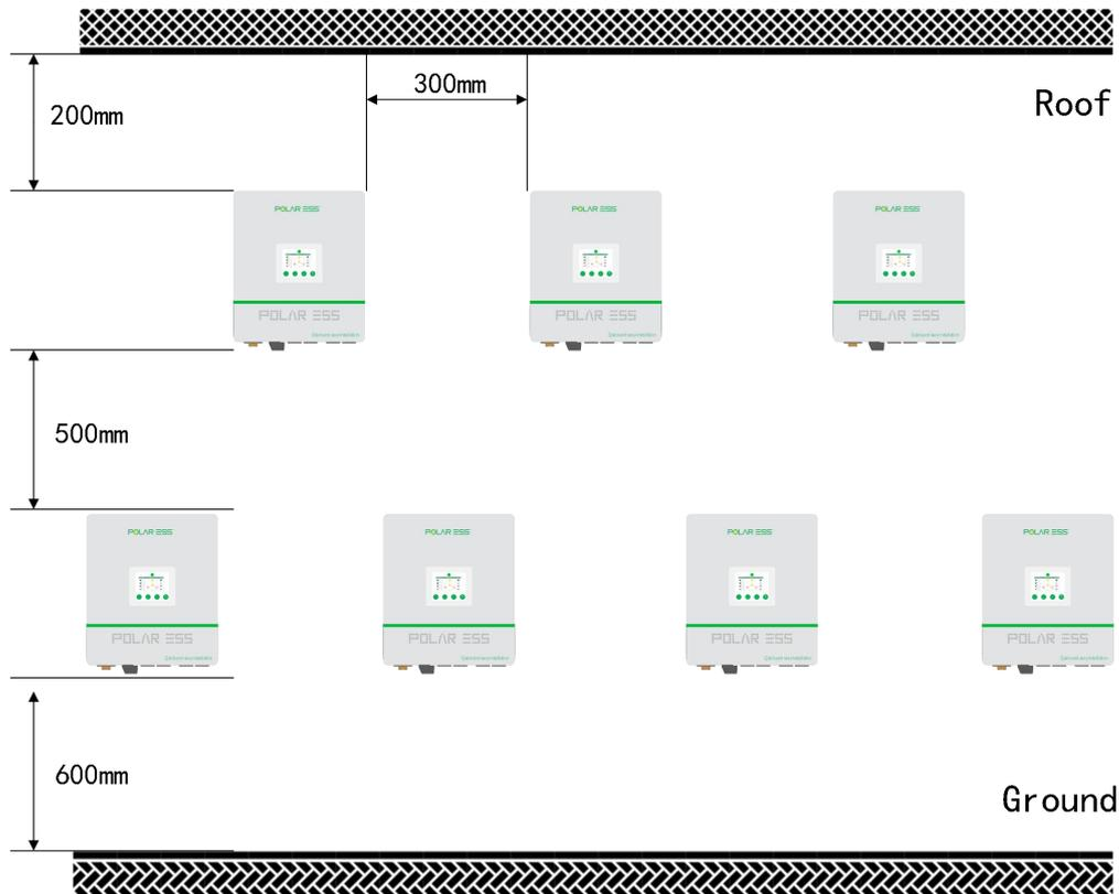
Ambient Dimensions Using Inverters in Series:
