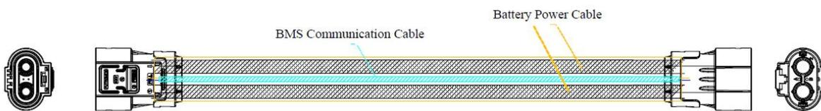
It integrates battery power cables and communication cables between the battery and inverter, so there is no need for additional battery communication cable connections.
