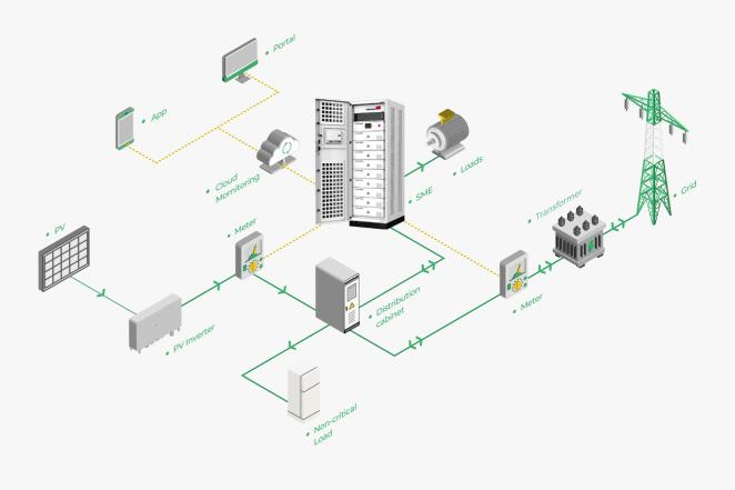
The PCS, battery pack, BMS, EMS, air conditioning, and fire protection are within a compact cabinet.
